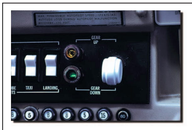
Figure 11-7. Typical landing gear switches and position indicators.
