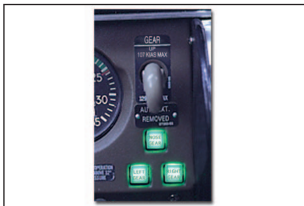
Figure 11-6. Typical landing gear switches and position indicators.
